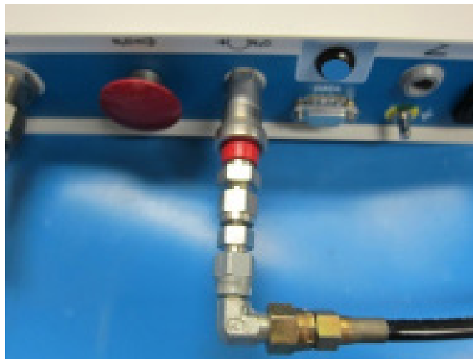
FIGURE 5: N 2 O INLET CONNECTION
