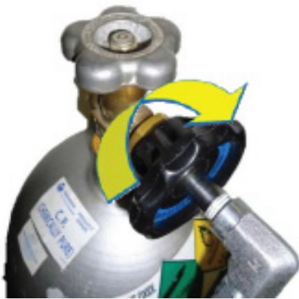
FIGURE 6: ATTACH BLACK KNOB TO THREADED CONNECTION
