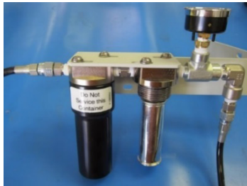
FIGURE 25: DESICCANT FILTER CARTRIDGE REMOVAL
