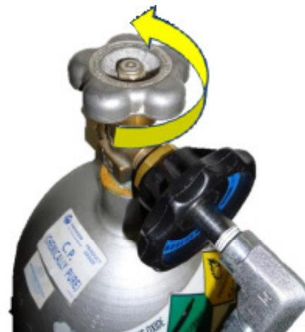
FIGURE 7: TURN VALVE COUNTER-CLOCKWISE TO OPEN
