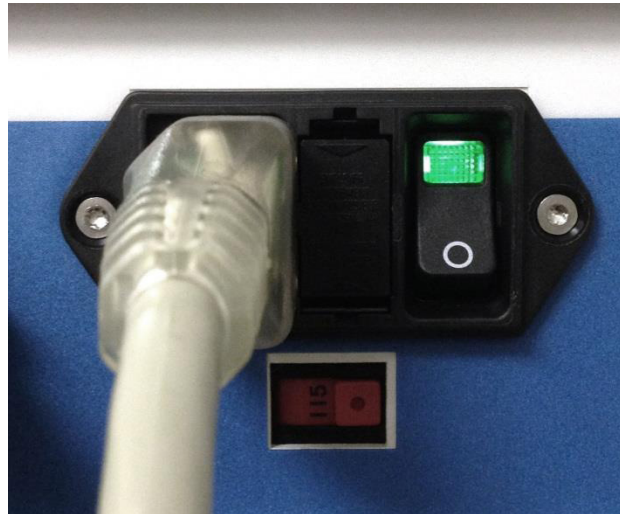
FIGURE 11: TURN-ON ATRICURE cryoICE BOX WITH SWITCH
