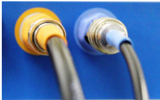
FIGURE 14: COLOR CODED PNEUMATIC CONNECTORS
