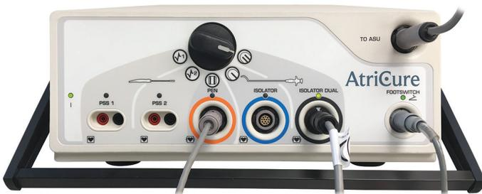
Note: Example shows ASB configured to power an Isolator® Synergy™ Clamp or Isolator Synergy Access® Clamp that is plugged in to the “Isolator Dual” channel.
