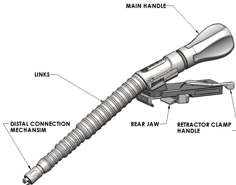
Figure 1 – Hercules Device
