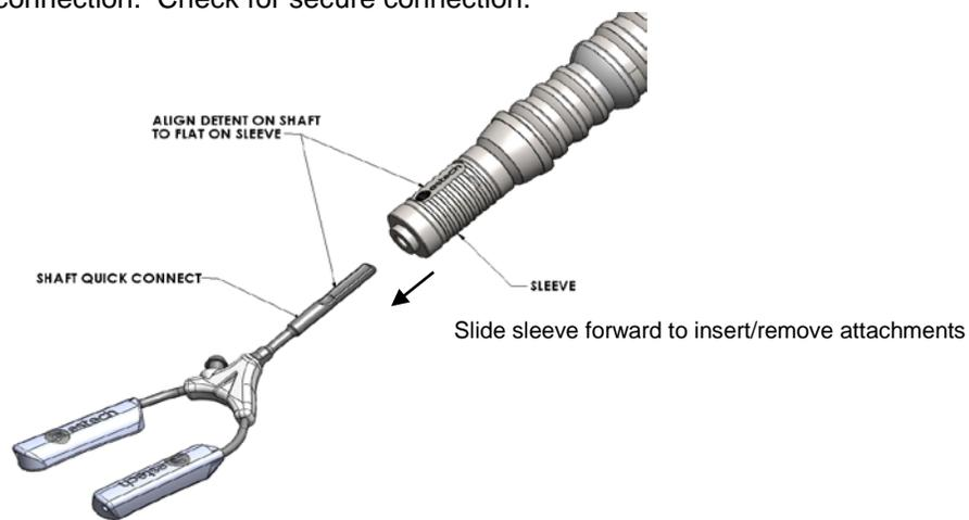
Figure 2 – Hercules 3 Quick Connect (401-161)
