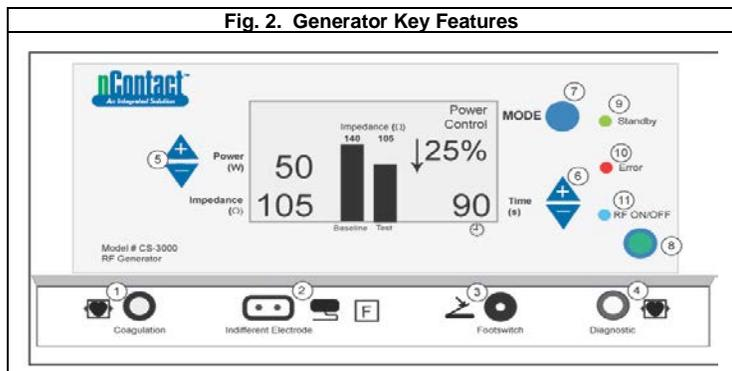
**(1) CSK-2030 Cable Connection; (2) Indifferent, Dispersive Electrode Connection; (3) Footswitch Connection; (4) Diagnostic Device Connection; (5) Power Adjustment; (6) Time Adjustments; (7) Mode button; (8) RF ON/OFF Button; (9) Standby Mode ED; (10) Error LED; (11) RF LED;**
