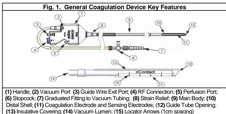
**(1) Handle; (2) Vacuum Port (3) Guide Wire Exit Port; (4) RF Connection; (5) Perfusion Port; (6) Stopcock; (7) Graduated Fitting to Vacuum Tubing; (8) Strain Relief; (9) Main Body; (10) Distal Shell; (11) Coagulation Electrode and Sensing Electrodes; (12) Guide Tube Opening; (13) Insulative Covering; (14) Vacuum Lumen; (15) Locator Arrows (1cm spacing)**
