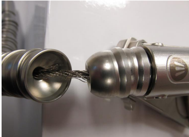
Cable demonstrating fatigue and fraying – Return to Estech
