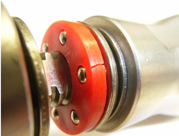
Broken or missing nylon washer – Return to Estech
