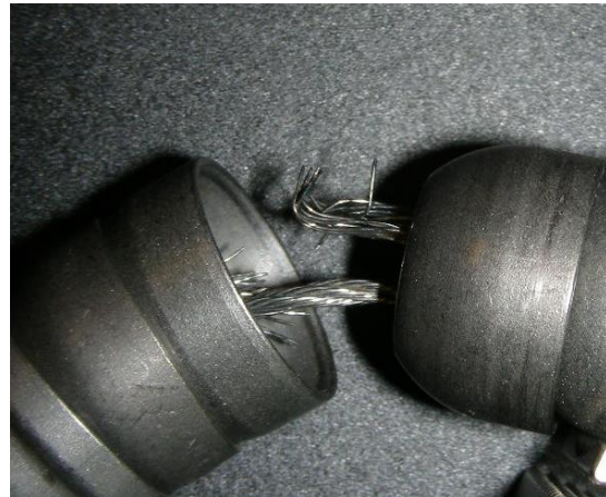
Appearance of a fraying cable – Do not Use
