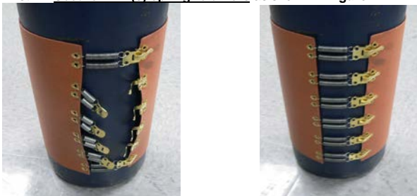
Figure 2 – Secure spring retainers, top and bottom retainers first.
